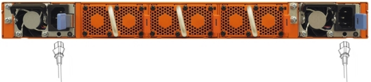
Figure 10 Connecting AC Power on a GigaVUE-TA200
