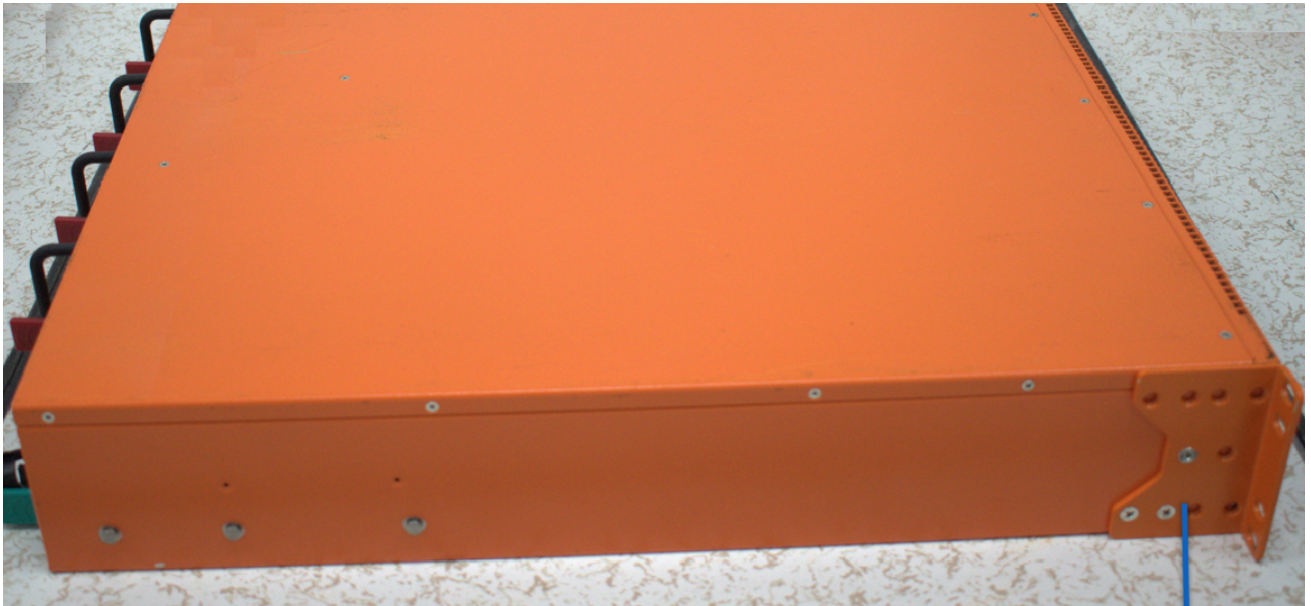
Front-Mounting Rack Ears In this picture, the rack ears are attached facing towards the front of the chassis.
